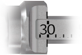
Two etch lines on the depth gauge sleeve indicate a 30mm measurement
