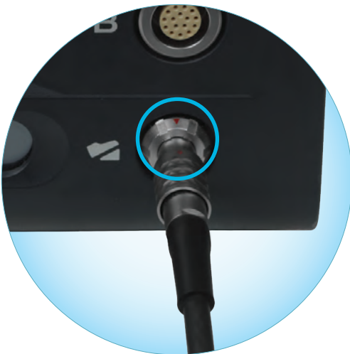
Red markings aligned on cable end and connector
