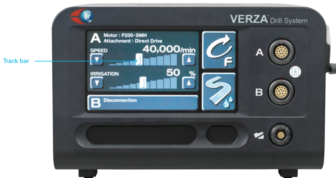
Touchscreen example displaying Motor A speed setting and irrigation flow rate
