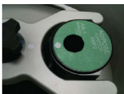
Figure 2: White dots facing the center of the rotor
