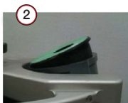
Figure 3: Adapter seated correctly (1) and adapter seated incorrectly (2)
