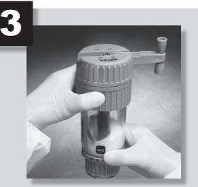
Attach cap to mixing chamber and tighten lower half firmly. Crank handle should be in the fully extended position
