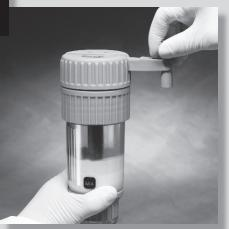
At 20 seconds, mix for 60 seconds, alternating 3 clockwise and 3 counterclockwise revolutions. Mixing speed should be one turn per second
