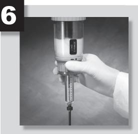
Attach angled delivery tube Rotate collar clockwise until it locks in the "LOAD SYRINGE" position
