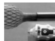
Figure 4: The release button is partially retracted, which begins to uncover the implant tail.
