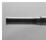
Figure 2: Detail of the distal end of the inner and outer hypotubes. The inner hypotube has a flared distal end and slightly reduced outer diameter.
