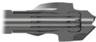
Reamer Shaft engaged with Reamer Head - cross-section view
