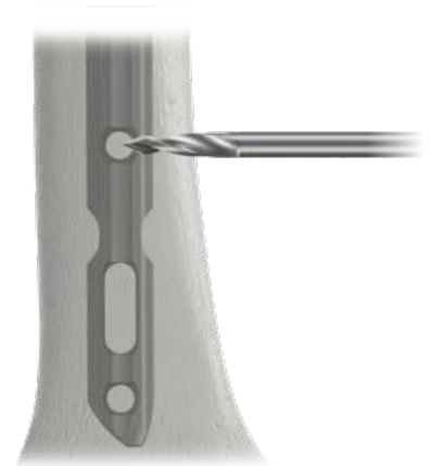
Identifying drill start point
