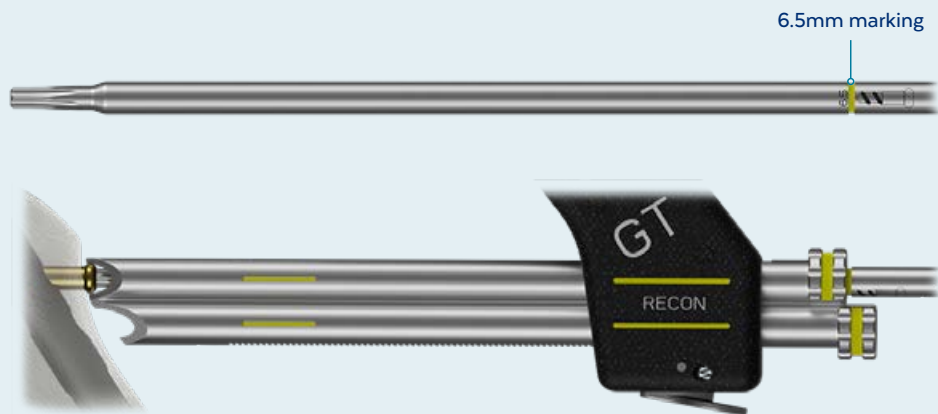
Final placement of 6.5mm Recon Screw shown
