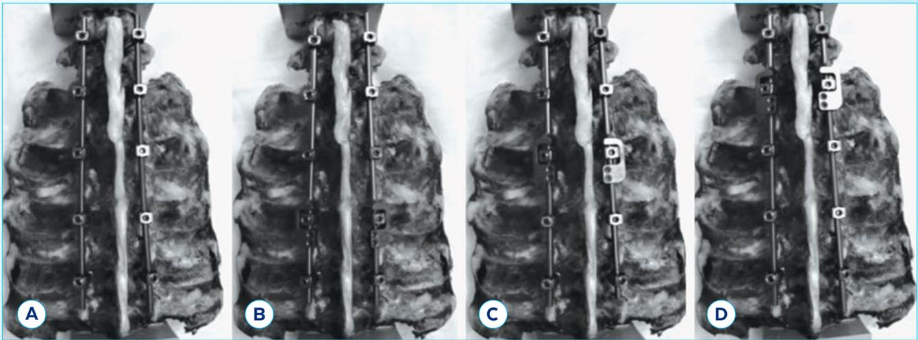
(A) Bilateral pedicle screw (BPS) T13-L4, (B) BPS L3-L4+integrated clamp (IC) T13-L3, (C) BPS L2-L4+IC T13-L2, and (D) BPS L1-L4+IC T13-L1.
