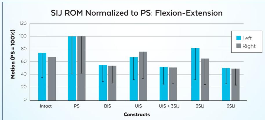
Mean ROM in the left and right SIJs in FE for all operative constructs, normalized to the PS construct.
