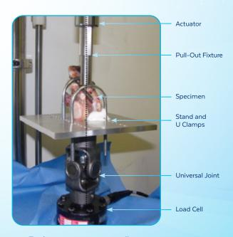
Testing setup to measure pull-out strength (MTS Mini Bionix III)
