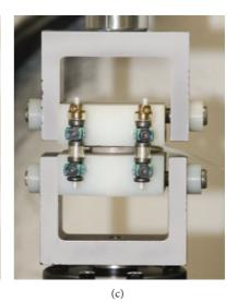
FIGURE 2: Testing constructs loaded in fixtures. Left to right: rigid rods, PEEK rods, and posterior dynamic stabilization. The pressure film can be seen above the spacer.
