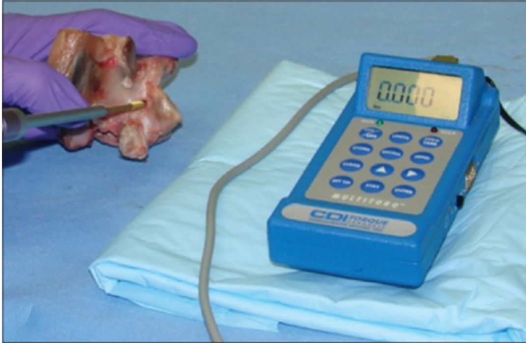
Torque meter used to measure insertion torques of pedicle screws
