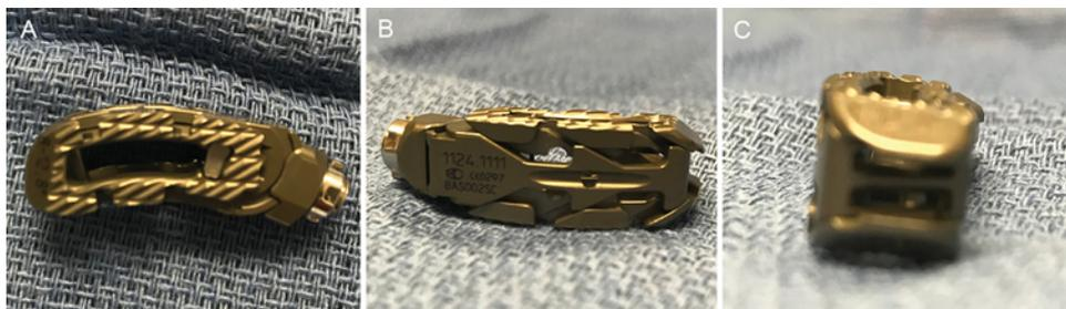
**FIG. 1.** Photographs of the Altera cage—this is a 31-mm length × 10-mm width, 15° lordotic cage expanded to 13 mm. **A:** Top-down view illustrates graft window and cage footprint. **B:** Front view of the cage shows the expansion mechanism. **C:** Lateral view illustrates the lordotic angle built into the cage.
